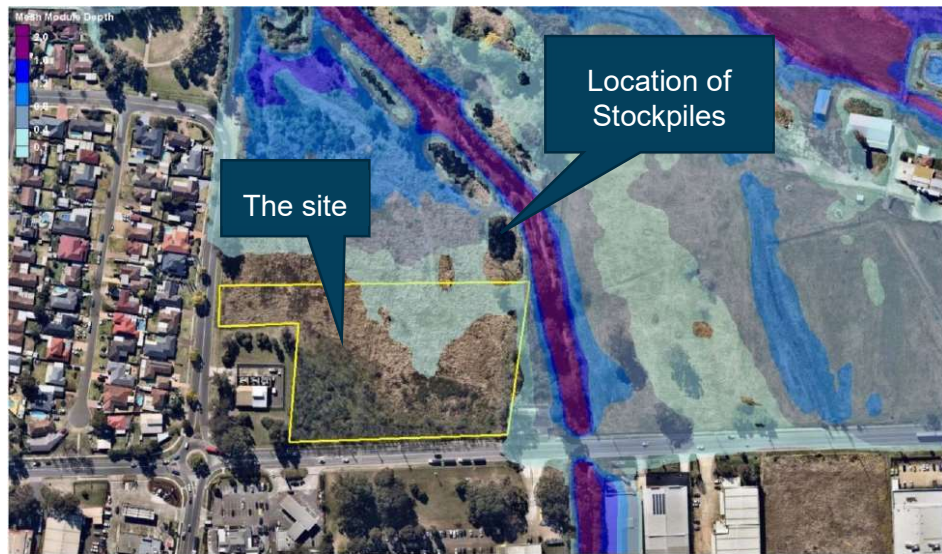
Figure 10 – Pre-development flood mapping
